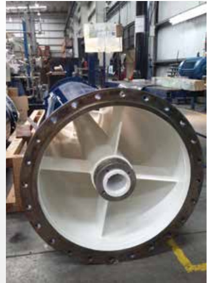
Pipe sections with Vesconite Hilube bushings.
