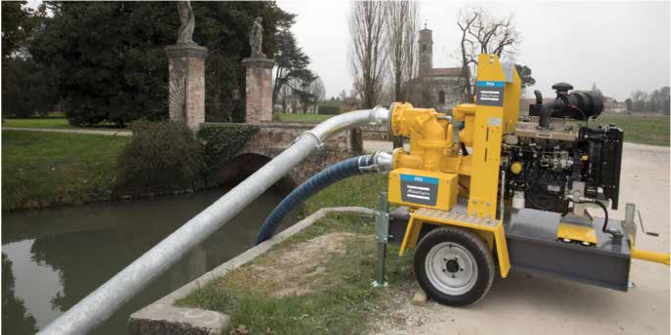
The operating flow range of centrifugal pumps is typically between 50 to 830 m 3 /h.
