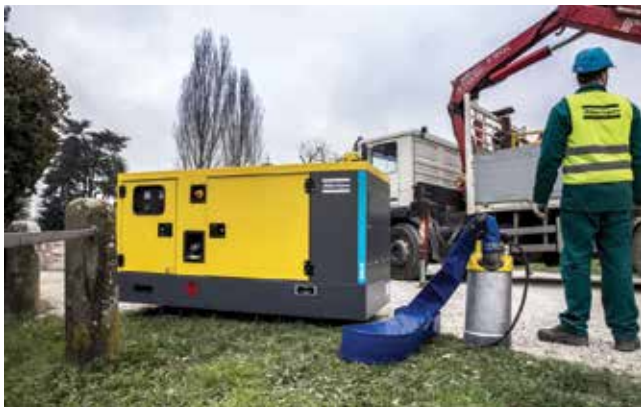
Electric submersible dewatering pumps offer portability & easy handling.
