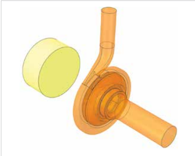
Figure 2: CAD model of the pump with flow volume (orange) and rotating zone (yellow).
